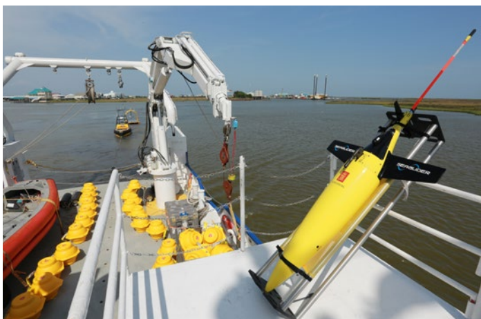
LADC-GEMM passive acoustic monitoring fleet (EARS buoys, gliders, and autonomous surface vehicle) on the way to collect over 30 Terabytes of data for scientists to analyze. Photo Credit: LADC-GEMM
