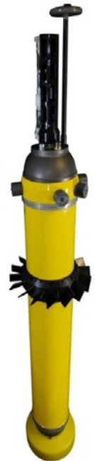
Photo Caption: An APEX-EM Float with an Optode Dissolved Oxygen Sensor at the top along with an Iridium antenna manufactured by Teledyne-Webb. The fins allow the profiler to rotate with depth to measure the two-dimensional currents. Photo Credit: Nick Shay.
