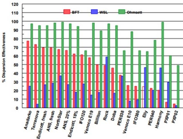
Figure 7. Synthesis of dispersant tests performed using various protocols (SL Ross Environmental Research, 2010)
