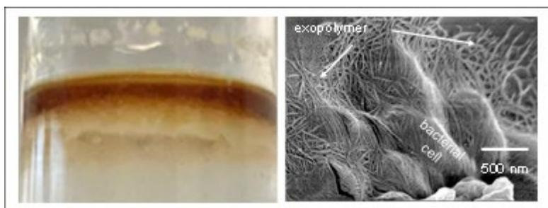
Figure 4 Bacterial growth at a pristine flat oil-water interface. On the right is a high resolution cryo scanning electron micrograph of cells and biofilm. From Omarova et al. (2018)
